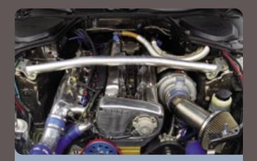
The ORC/Top Secret D1GP Fairlady Z uses the classic RB26DETT to deliver reliable high horsepower while going sideways. Amazingly, Top Secret has installed the RB further back and lower in the engine bay than the stock VQ engine. With excellent weight distribution and over 700hp coming from a mildly tuned RB, expect this Z to do extremely well in the D1GP for 2005. For more information visit www.oguraclutch.co.jp.
